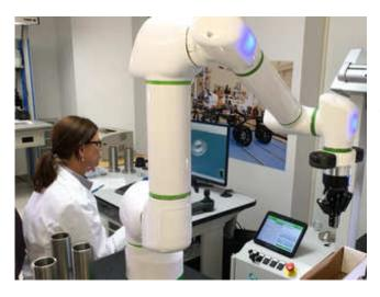
Cobots – short for Collaborative Robots – differ from traditional industrial robots in that they have engineered safety features to limit force and speed. Thanks to these safety features, OB7 can be deployed without fencing or physical barriers; OB7 can work together with a human operator, as an assistant.
