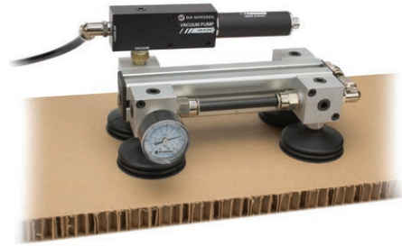
NVP80-200M distributes vacuum to four cup mount/manifold assemblies to pick up corrugated board.
